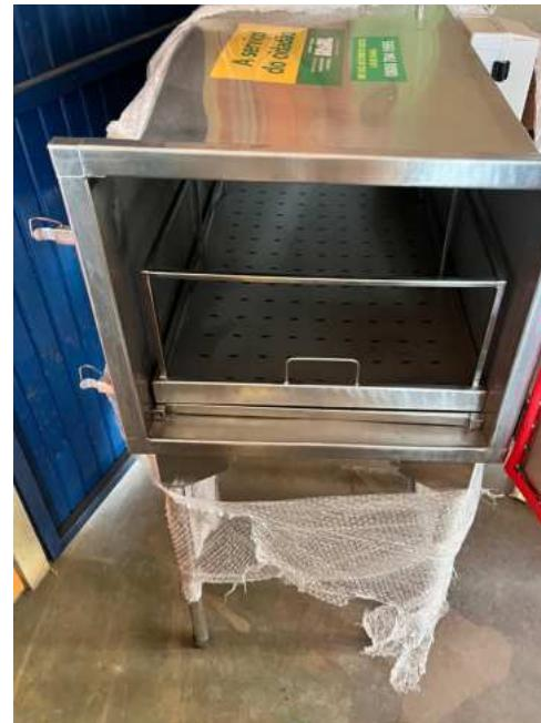
**DESCRISTALIZADOR DE MEL A SECO, TIPO ESTUFA, 4 BALDES, MARCA ASCINOX –
